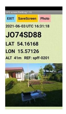
**GPS position** —a very useful tool for creating documentation of field work. Use the Photo button to launch the built-in camera app, take a photo to add it to the GPS data and save it as a file in the log directory.
